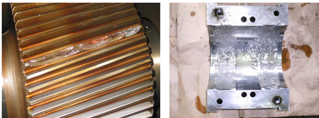
Fig. 6. Failer on: a) tooth of the gear-wheel, b) bearing ring.
