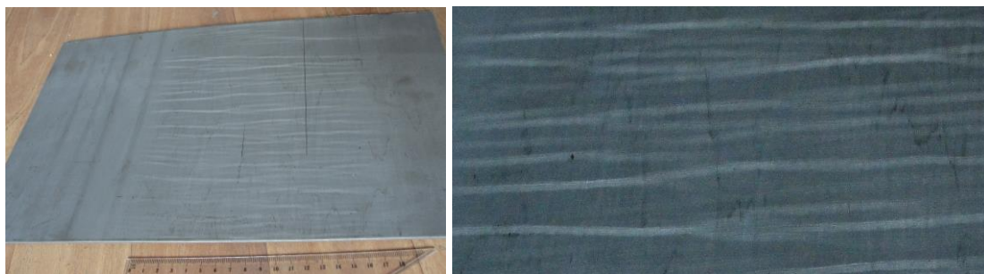
Fig. 2. Coil breaks in low carbon steel sheet.
