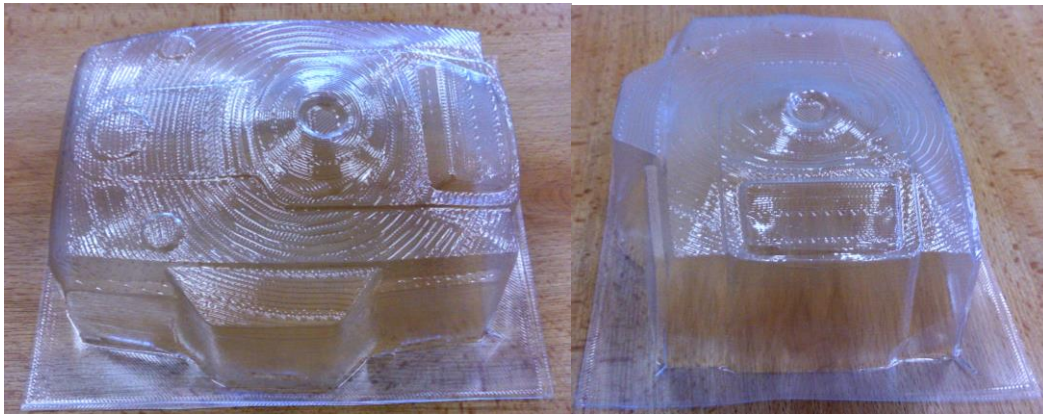
Fig. 3 Lid made from PET foil on FDM mold
