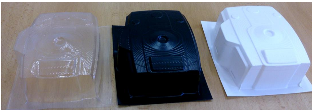
Fig. 4 Lid made from PET(left) and HIPS foil on FDM mold
