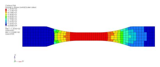
Figure 5: Finite element result of the miniature specimen to check the stress conntration.
