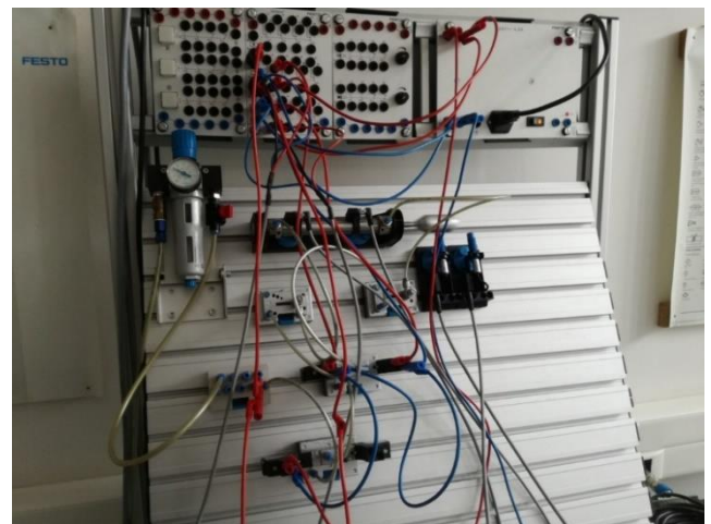
Fig. 3 a., the pneumatic and electric scheme of the test system; b., the built test system
