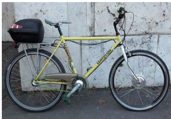
Fig. 1. One of the human-electric hybrids used in the experiment. The 250W engine is built in the front wheel the battery is in the box above the rear wheel.
