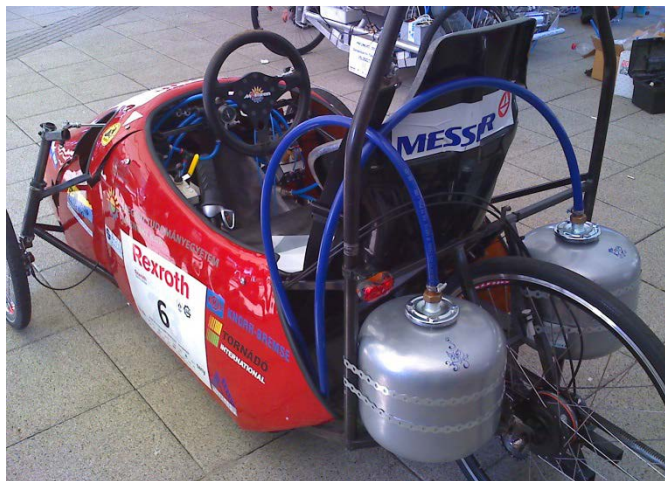
Fig. 3. First buffer tanks
