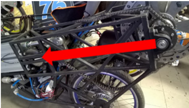
Fig. 4. Direction of load on the engine frame
