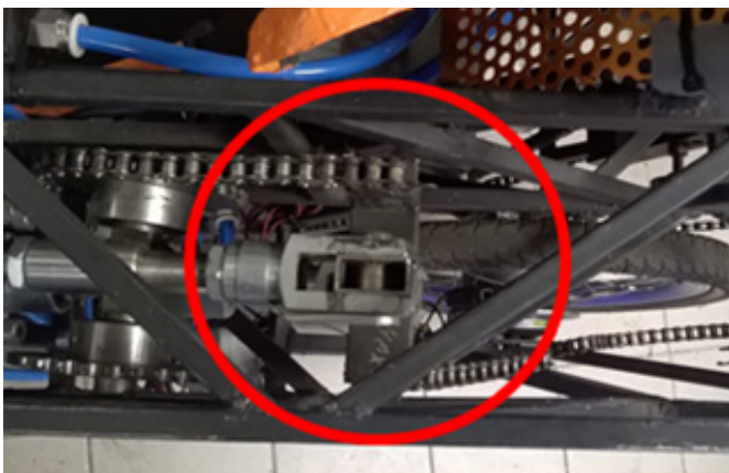
Fig.5. Chain break as a result of chassis distortion
