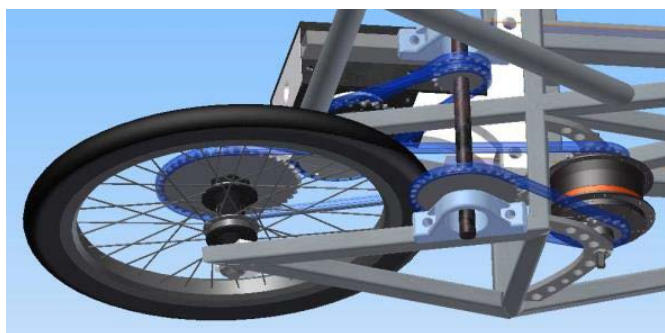
Fig. 6. Drivechain of the Diff-Air with the hub transmission in front of the wheel
