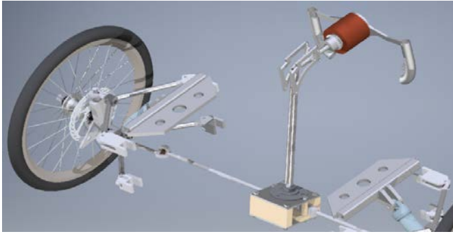
Fig. 8. The front running gear of the Airrari, 2016
